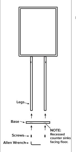
Insert screws into base and up into legs. NOTE: The side of the base with the recessed counter sink holes should be facing the floor. Use Allen wrench to fasten base to legs.
