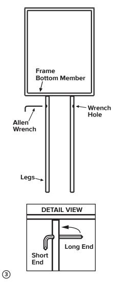
Insert long end of Allen wrench into wrench hole until seated. Use long end of Allen wrench as a lever and tighten leg (very tight). TIP: Hold the bottom member of frame with one hand and tighten leg with the other hand. Repeat for other leg.
